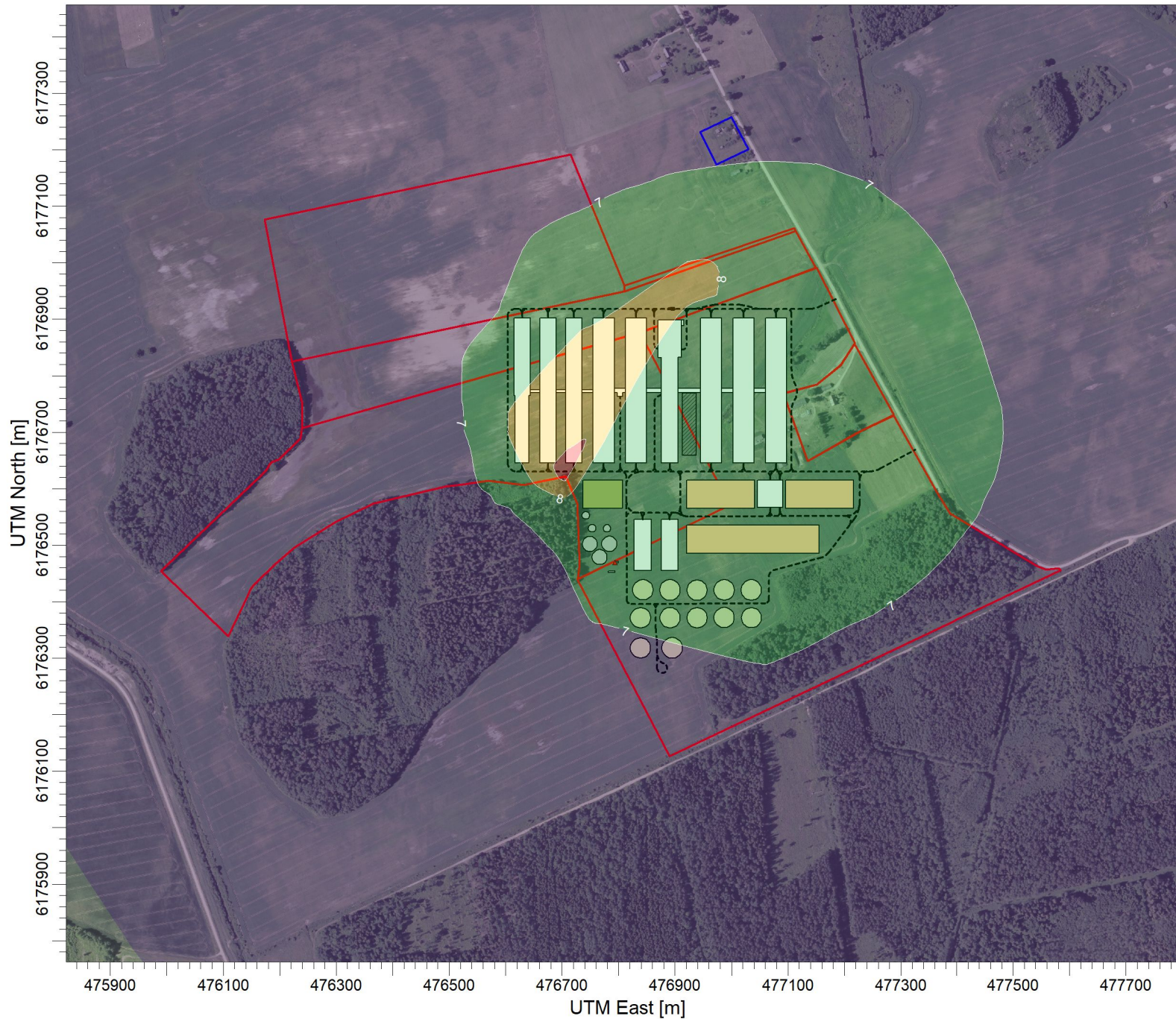
PLOT FILE OF ANNUAL VALUES AVERAGED ACROSS 5 YEARS FOR SOURCE GROUP: ALL Max: 9,2 [ug/m^3] at (476704,45; 6176621,09)
