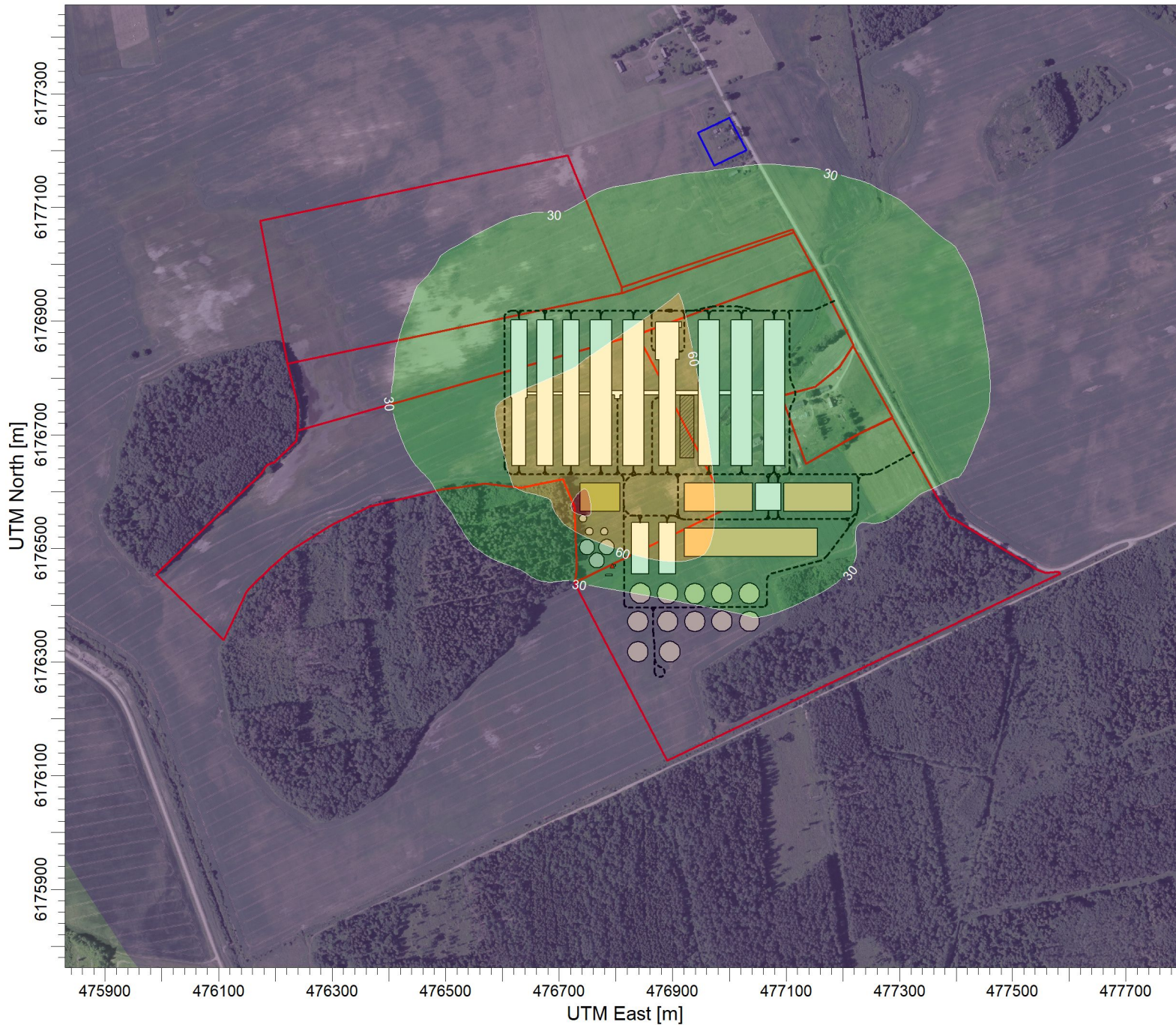
PLOT FILE OF 98.50TH PERCENTILE 1-HR VALUES FOR SOURCE GROUP: ALL Max: 94,1 [ug/m^3] at (476726,32, 6176568,24)
