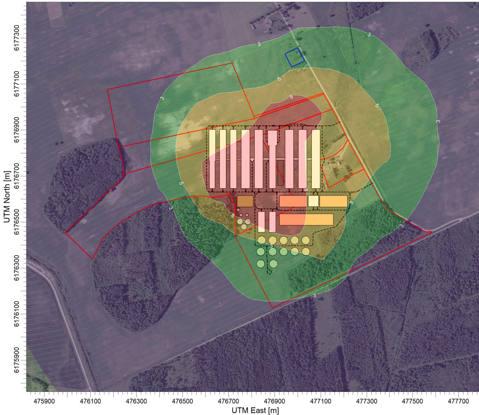
PLOT FILE OF 98.08TH PERCENTILE 1-HR VALUES FOR SOURCE GROUP: ALL Max: 13,8 [OU/M**3] at (476726,32, 6176568,24)
