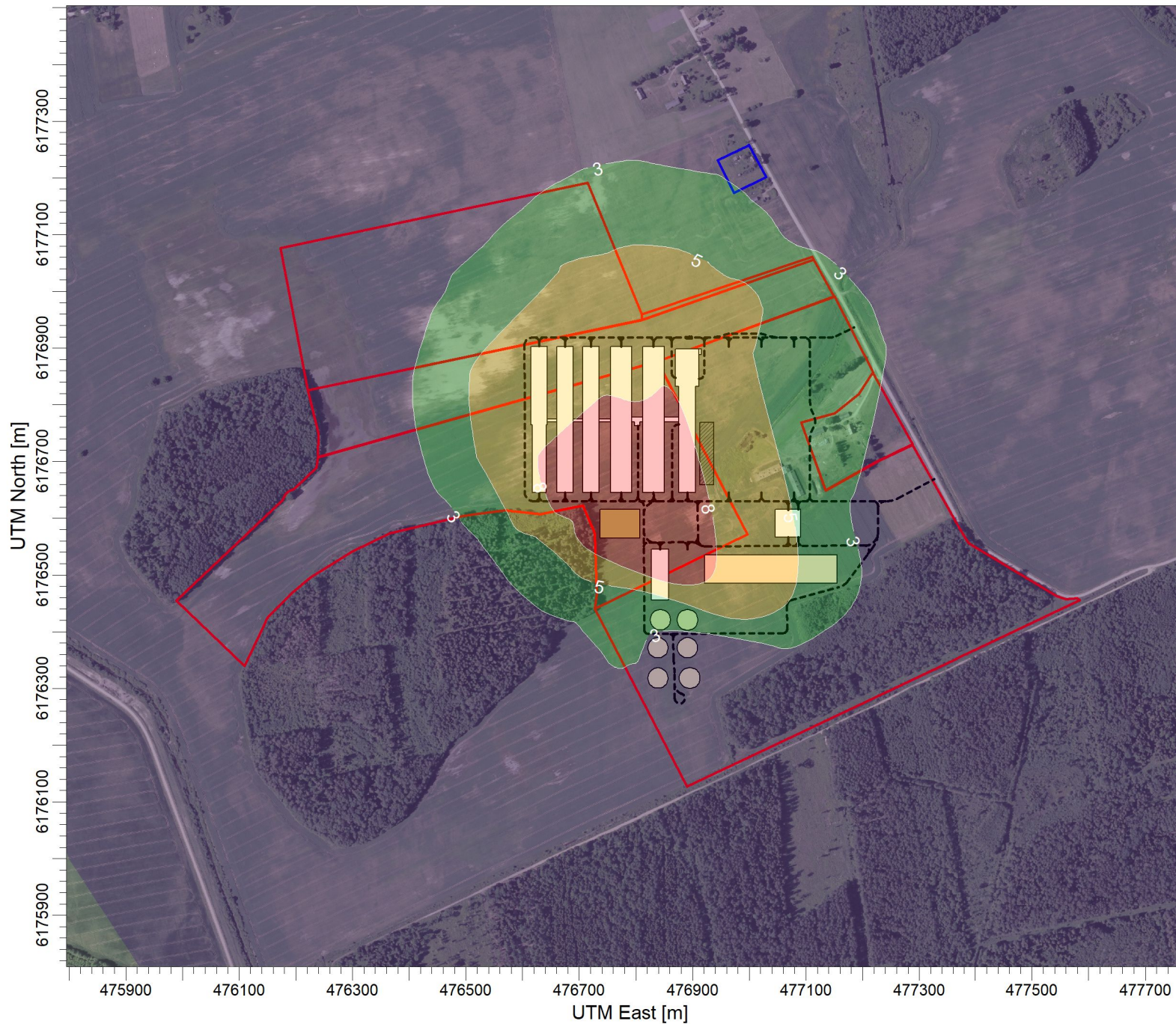
PLOT FILE OF 98.08TH PERCENTILE 1-HR VALUES FOR SOURCE GROUP: ALL Max: 12,7 [OU/M**3] at (476726,32, 6176568,24)
